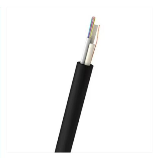
The ASU Cable is a self-sustaining optical fiber solution designed for connecting devices in both urban and rural network deployments. Recommended for spans of 80-120 meters, this fully dielectric cable features an FRP strength member for traction while eliminating electrical arcing risks. Its user-friendly design simplifies installation by removing the need for stringing or grounding procedures.
