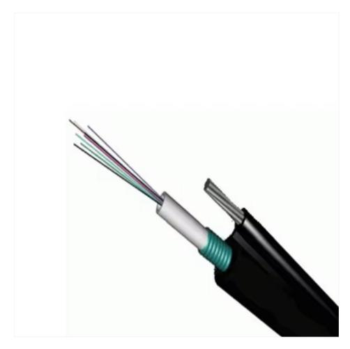
The GYXTC8S cable is constructed by inserting a 250µm fiber into a loose tube made of a high-modulus material filled with a water-repellent compound. The loose tube is coated with a double-sided plastic coated steel strip (PSP) longitudinally, and a water-blocking material is added between the steel strip and the loose tube to ensure compact and longitudinal water blocking of the cable, with the steel strand integrated into an 8-shaped type inside the polyethylene sheath.
