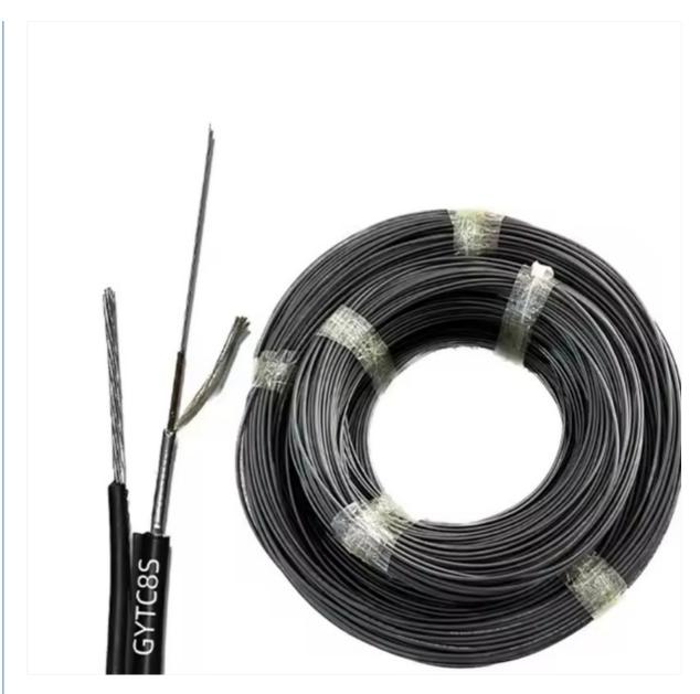
The cable features a figure-eight design with a metallic strength member constructed from stranded wires, protected by a polyethylene sheath. Additional protection comes from corrugated steel tape armor and a polyethylene outer sheath, providing exceptional crush and bullet resistance.
