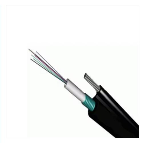
The GYXTC8S cable features a 250µm fiber core encased in a high-rigidity flexible tube with water-repellent gel. The tube is wrapped with plastic-coated steel tape (PSP) for longitudinal water protection, combined with water-blocking material between layers. The 8-shaped steel strand provides structural support, all protected by a durable polyethylene sheath.
