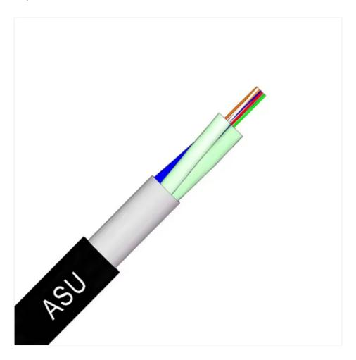
The ASU Cable is a Self-Supported Optical Cable designed for inter-device connectivity, recommended for urban and rural network installations with spans of 80 or 120 meters. It incorporates an FRP strength member for tension, which prevents electrical discharges, and is simple to handle and install without the need for strings or grounding.
