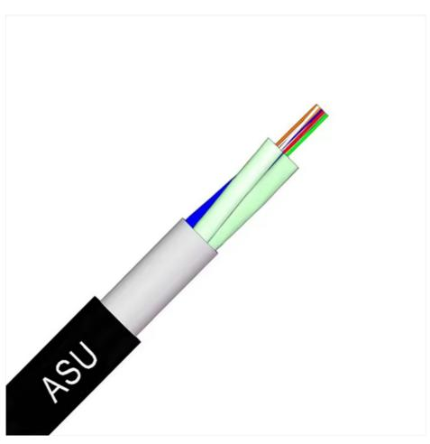
The ASU Cable is a Self-Supported Optical Cable designed for both urban and rural network installations, available in lengths of 80 or 120 meters. Its FRP strength member serves as a non-conductive load-bearing component, preventing electrical discharges. The cable's design eliminates the need for guy wires or grounding, making installation straightforward and efficient.
