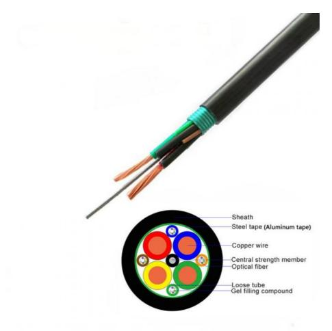
Provides equipment power and signal transmission in a single cable
