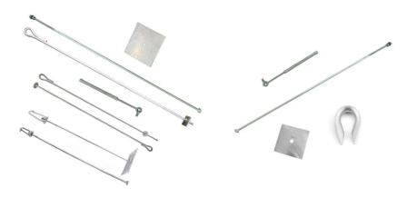
This stay rod is used to connect the stay wire to the ground anchor, also known as the stay set. It ensures that the wire is firmly rooted to the ground and everything remains stable. There are two types of stay rods available in the market: the bow stay rod and the tubular stay rod. The difference between these two types of power-line accessories is based on their designs.
