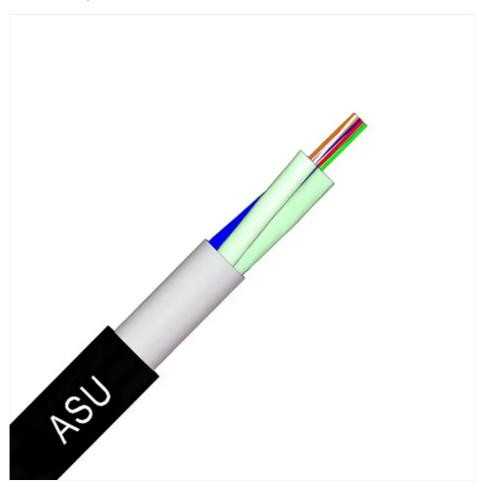
The ASU Cable is a Self-Supported Optical Cable tailored for connecting devices, suitable for both urban and rural networks with lengths of either 80 or 120 meters. It features an FRP strength member to assist with traction, preventing electrical discharges, and is designed for straightforward installation without the necessity for guy wires or grounding.
