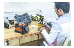
02 Attenunation test for each fiber by OTDR after production,and QC for every detail
