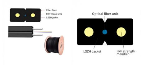
The fiber optic drop wire unit is situated in the middle, surrounded by two parallel steel wires. The cable is encased in a black or colored LSZH sheath. FTTH stands for Fiber to Home and is constructed with 2\*0.5mm FRP for self-supporting capability.
