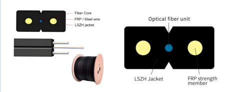
At the center, you will find the fiber optic drop wire unit, with parallel steel wires on both sides. The cable is protected by a black or colored LSZH sheath. FTTH, or Fiber to Home, utilizes a self-supporting design featuring 2\*0.5mm FRP.
