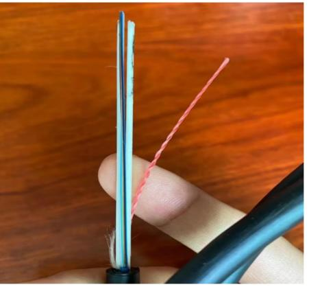
ASU cable is one loose tube stranded. Fibers, 250um, are positioned into a loose tube made of high modulus plastics. Two FRP (Fiber Reinforced Plastic) as as strengthen member. Cable surface is extruded with HDPE (polyethylene) sheath. Designed for spans ranging from 80 to 120 meters, it provides low attenuation and high signal speed. Ideal for optimizing data transmissions in outdoor areas.
