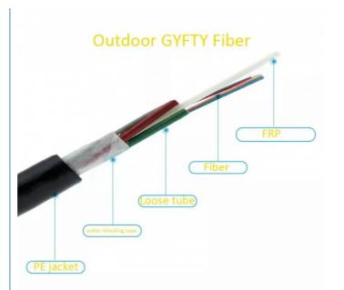
In the GYFTY cable, single-mode/multimode fibres are positioned in the loose tubes, which are made of high modulus plastic materials, while the loose tubes strand together around non-metallic central strength member (FRP) into a compact and circular cable core. For certain high fibre count cables, the strength member would be covered with polyethylene (PE). The water-blocking materials are distributed into the interstices of the cable core. Then the cable is completed with a PE sheath.
