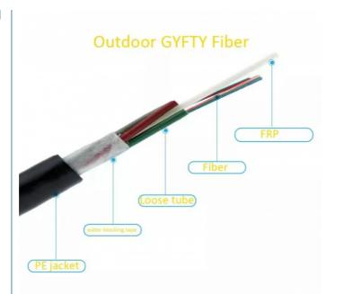
The 2-288 fibers are positioned in PBT loose tubes filled with gel. Tubes (and fillers) are stranded around the non-metallic strength member (FRP) to form the cable core. Then the cable core is filled with the cable jelly to protect it from water penetration. Finally a PE jacket is extruded.
