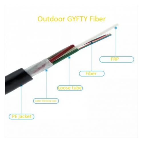
In the GYFTY cable, single-mode/multimode fibers are positioned in high modulus plastic loose tubes that strand around a non-metallic central strength member (FRP) into a compact, circular cable core. For high fiber count cables, the strength member is covered with polyethylene (PE), with water-blocking materials distributed in the cable core interstices.
